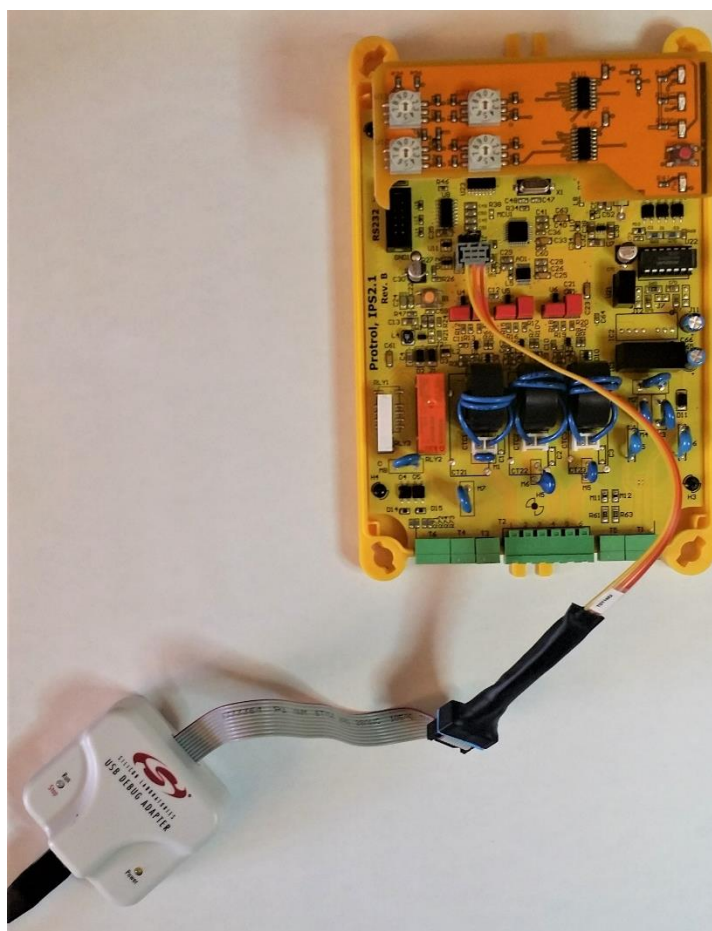
Figure 16. USB Debug Adapter connected to IPS2.
